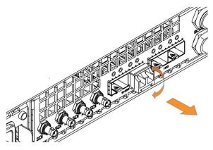
The SFP module should be removed from the generator while the instrument is being transported.
