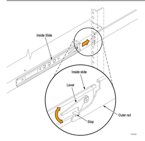
2. Push the instrument into the rack until it stops.
