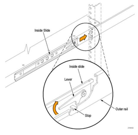
4. Pull the instrument past the stops and out of the rack.
