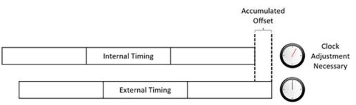
When the external reference is restored, the SPG9000 finds the actual offset between its internal clock to the reference source. The SPG9000 then goes into holdover recovery
