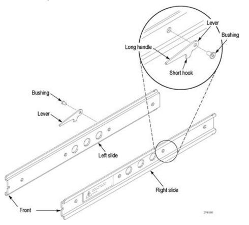
The example shows how to attach the slide levers for the SPG9000 instrument.
