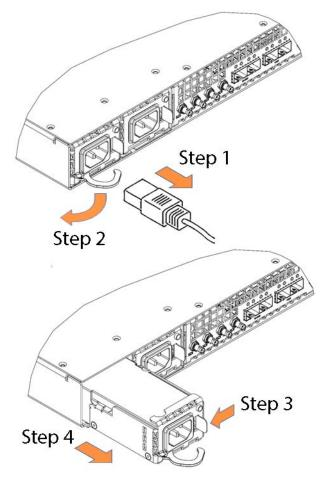
2. Pull out the handle located at the bottom of the supply.
