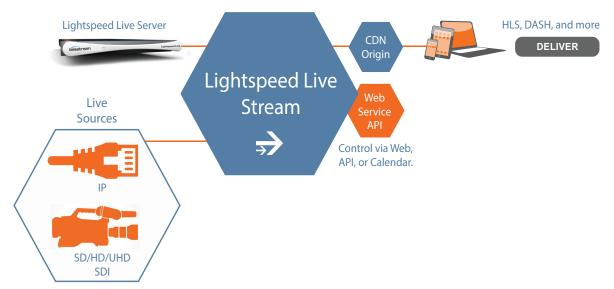
Lightspeed Live Stream runs exclusively on Telestream's *Lightspeed Live Server*. Lightspeed Live Stream servers can be joined together to create a multi-server streaming group. The Telestream Live Service is configured, operated, and controlled via the Live Stream web application, and a REST API is also provided for integration and control by other systems.
