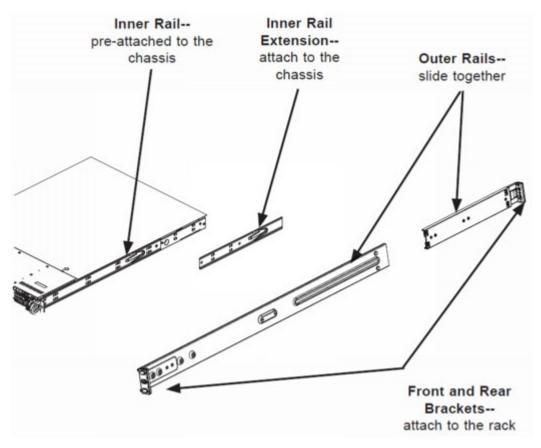
Align the extension holes with the hooks on the side rail and slide the extension forward to engage the hooks until the quick release bracket snaps into place. For added stability, you can secure the extension with a screw.
