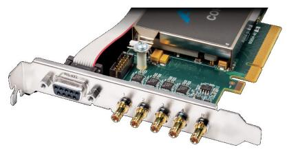
**Note:** The 4-port SDI card is inserted upside down into the rear panel at the bottom right corner. Refer to imprinted labels (1 2 3 4) and R for proper cable connection. The RS-422 port is unused.
