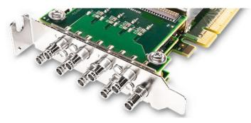
**Note:** Refer to imprinted labels (1 through 8) and R for proper cable connection.
