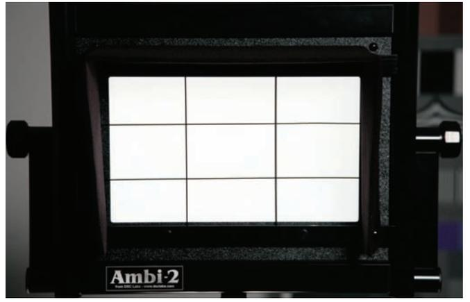
Figure 1b. Ambi Illuminator with grid over transparency.
