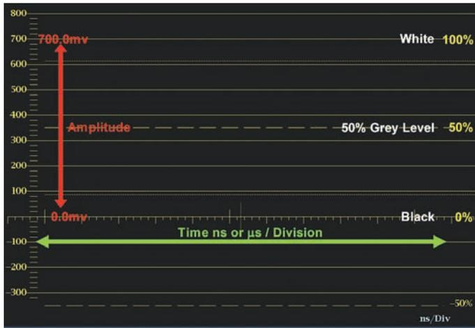
Figure 1a. Waveform display.
